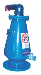
SPS air release valve incorporates a kinetic and an automatic air release valve in one single valve body. Each function in the sewage system is to release air (gases) and to admit air into sewage and waste water lines. The exclusive structure guarantees complete separation of the liquid from the sealing system and provides optimum working conditions.
